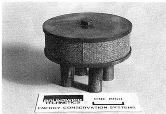
Fig. 2 Test apparatus: specimen holding fixture shown with cylindrical specimen
